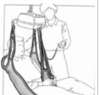
Raise the patient (up on hand control) and as raises check to ensure straps are firmly in place.
