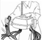
Attach the head sling loops to carry bar first, than leg straps to leg hooks.
